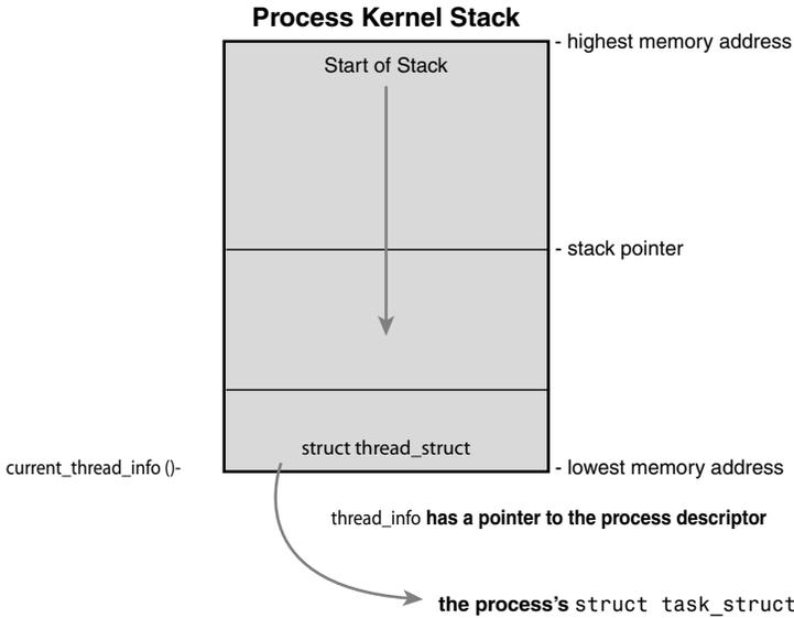
Figure 3.2 The process descriptor and kernel stack.
